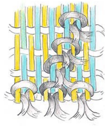
Alignment D. Tent band knotting with extra offsets ; knots arranged to make a steep diagonal.
